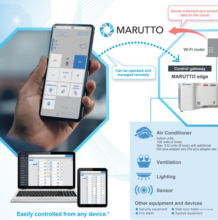
Interlocking with 3rd party systems Connectivity with other systems Connecting and interlocking with WAGO I/O system is possible by communication link. BACnet® compatible Option MARUTTO connects to 3rd party BMS and controllers via BACnet® \*Please contact your sales representative for communication specifications.
