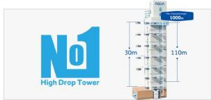
2 Allowable pipe length and height difference between Indoor and outdoor outdoor unit (outdoor unit above)
