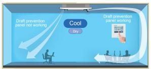
User can position panels by using the remote controller (RC-EX3A, Wireless kit) only when Draft Prevention Panel is available.
