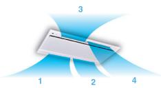
The flap can swing within the range of upper and lower flap position selected with wired control.
